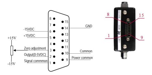
Figure 10. D07-11CM MFM- D Connector
