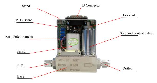
Figure 2. Structure of D07-11C
