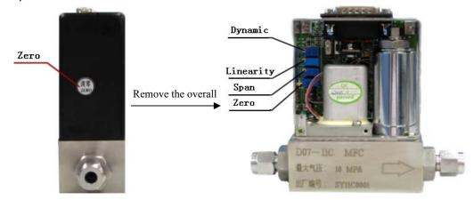
Figure 13. The position of potentiometer in 11C, 11CM, 11E
