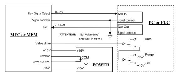
Figure 12. PC Directly Connection
