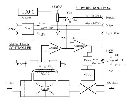
Figure 3. Operation Principle of MFC
