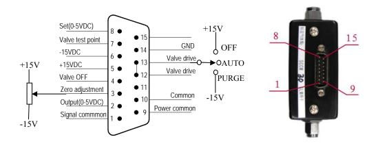
Figure 7. D07-11C D07-11E MFC "B" Connection
