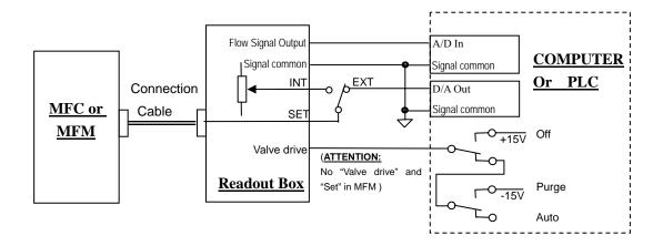
Figure 11. Connection with PC through Readout Box
