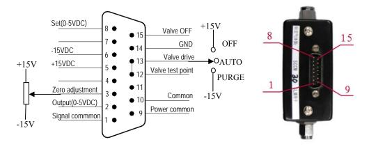
Figure 9. D07-11C D07-11E MFC "T" Connection
