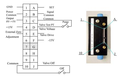
Figure 8. D07-11/ZM D07-12/ZM MFC Electric Connection
