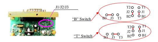
Figure 11. 12A MFC Socket Switch Connection (11A is same as this)
