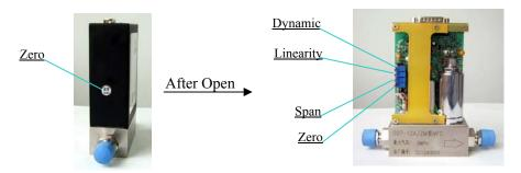
Figure 17. The position of potentiometer in 12A, 12AM(12,12M)
