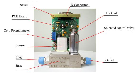
Figure 2. Structure of D07-12A
