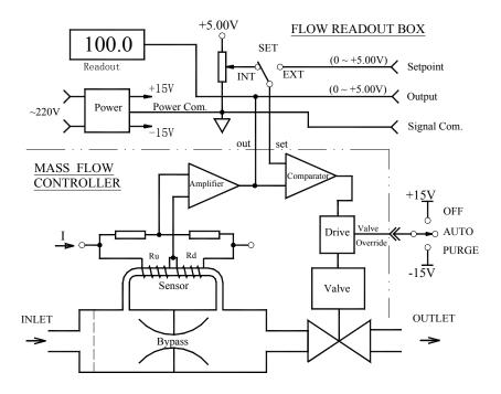
Figure 3. Operation Principle of MFC
