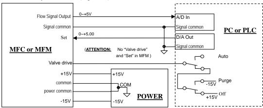
Figure 15. PC Directly Connection
