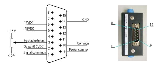
Figure 13. D07-11AM/ZM, D07-12AM/ZM MFM- D Connector
