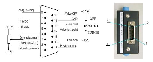
Figure 12. D07-11A/ZM, D07-12A/ZM MFC "T" Connection
