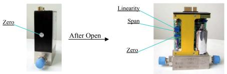
Figure 16. The position of potentiometer in 11, 11M(11A,11AM)
