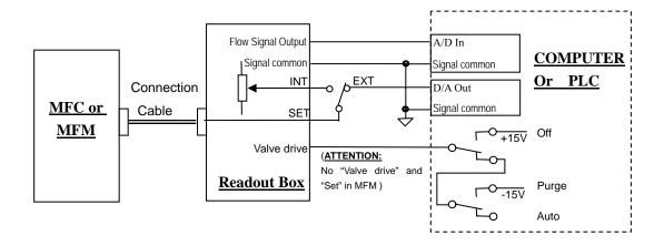
Figure 14. Connection with PC through Readout Box
