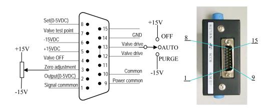
Figure 10. D07-11A/ZM, D07-12A/ZM MFC "B" Connection
