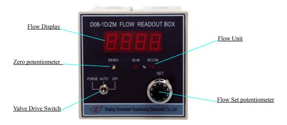
Figure 18. Flow Readout Box Operating Panel
