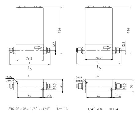
Figure 5. D07-11A/ZM, D07-11AM/ZM, D07-12A/ZM, D07-12AM/ZM
